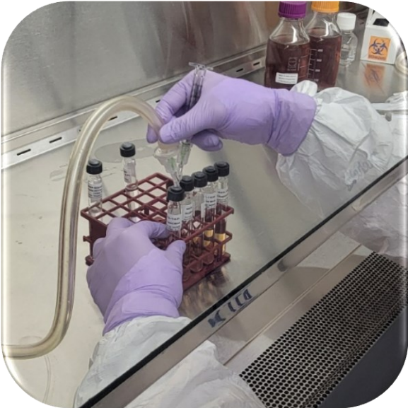
Gas exchange through a needle and syringe system
