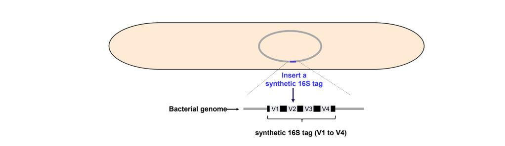
**Figure 2. Production of tagged strains.** ATCC created three unique synthetic 16S tag sequences mimicking the native 16S rRNA gene from 3 bacterial strains (*E. coli*, *C. perfringens*, and *S. aureus*). Each tag consists of 4 artificial variable regions (corresponding to V1 through V4 of the 16S rRNA gene) flanked by conserved regions for PCR amplification. Each tag sequence was integrated into the genome of their cognate strains to create three tagged strains.
