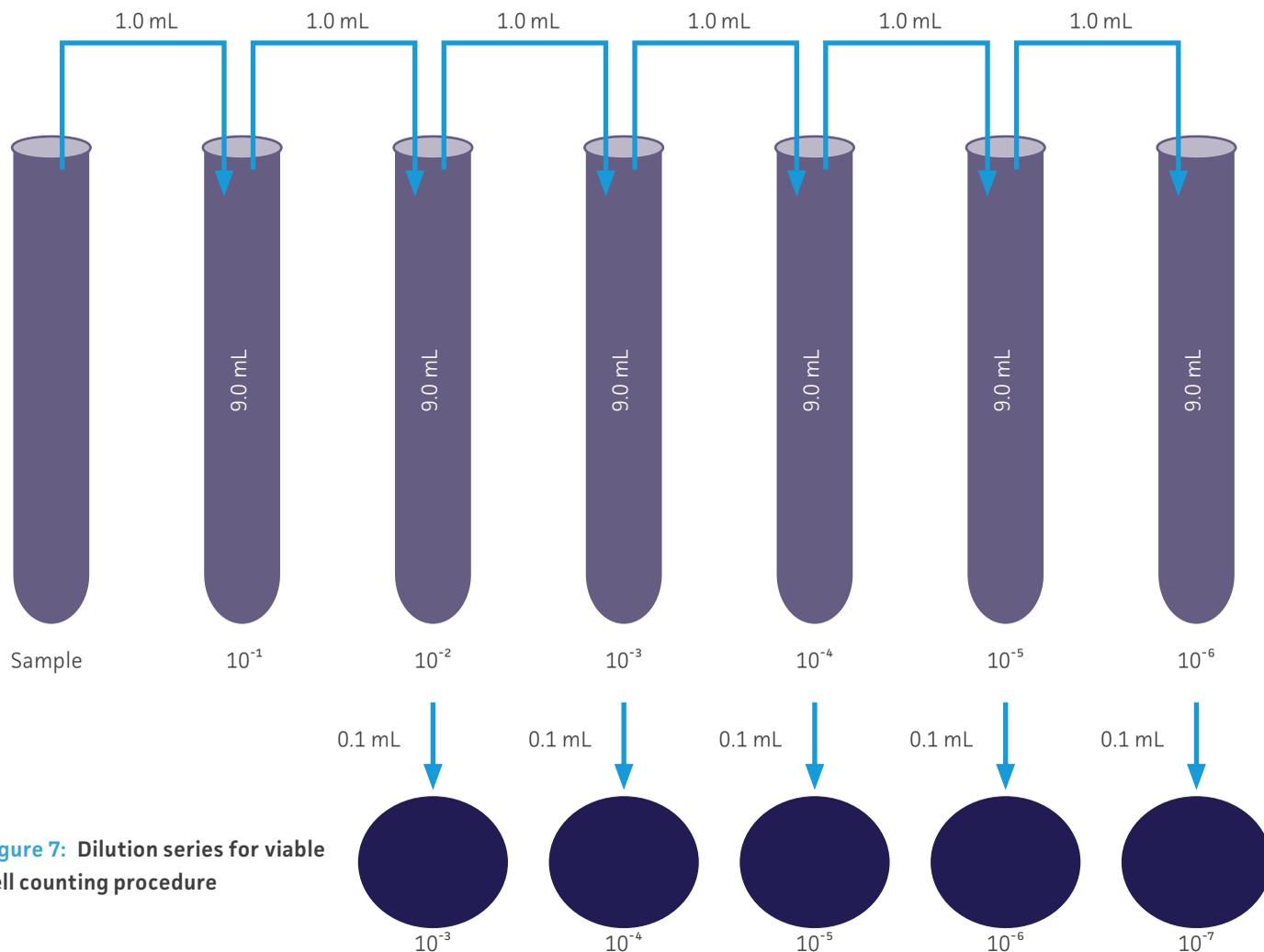
**Figure 7: Dilution series for viable cell counting procedure**
