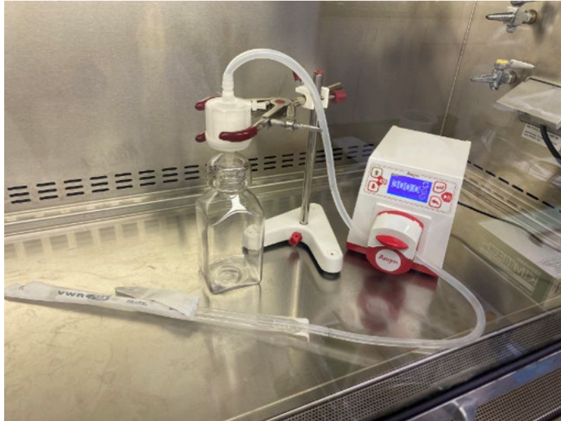
Figure 2: Peristaltic pump and harvest setup.
