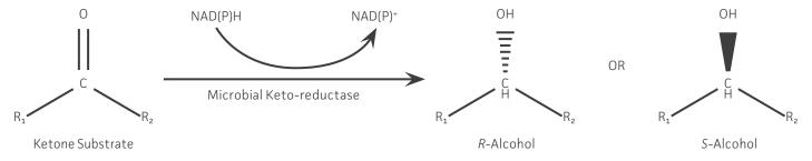
Figure 1: Representative keto-reductase reaction used in the asymmetric (ie chiral) synthesis of a secondary alcohol from a ketone. The substrate specificity (ie R groups that can be accepted) and the R or S stereochemistry of the alcohol product formed is determined by the enzyme's structure.
