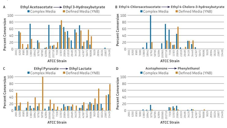
Figure 3: Conversion of Ethyl Acetoacetate (A), Ethyl 4-Chloroacetoacetate (B), Ethyl Pyruvate (C) and Acetophenone (D) to their corresponding alcohols by ATCC strains lyophilized in complex or defined media plus 10% (w/v) trehalose, stored at 4°C.
